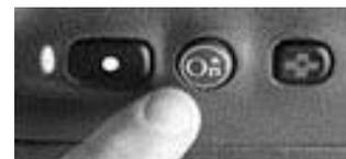
OnStar is a safety, security and information service, with a three-button user interface built into the vehicle (see photo).<sup>7</sup> OnStar uses the Global Positioning System (GPS) satellite network and embedded cellular technology to link the vehicle and driver to one of two OnStar service centers.
