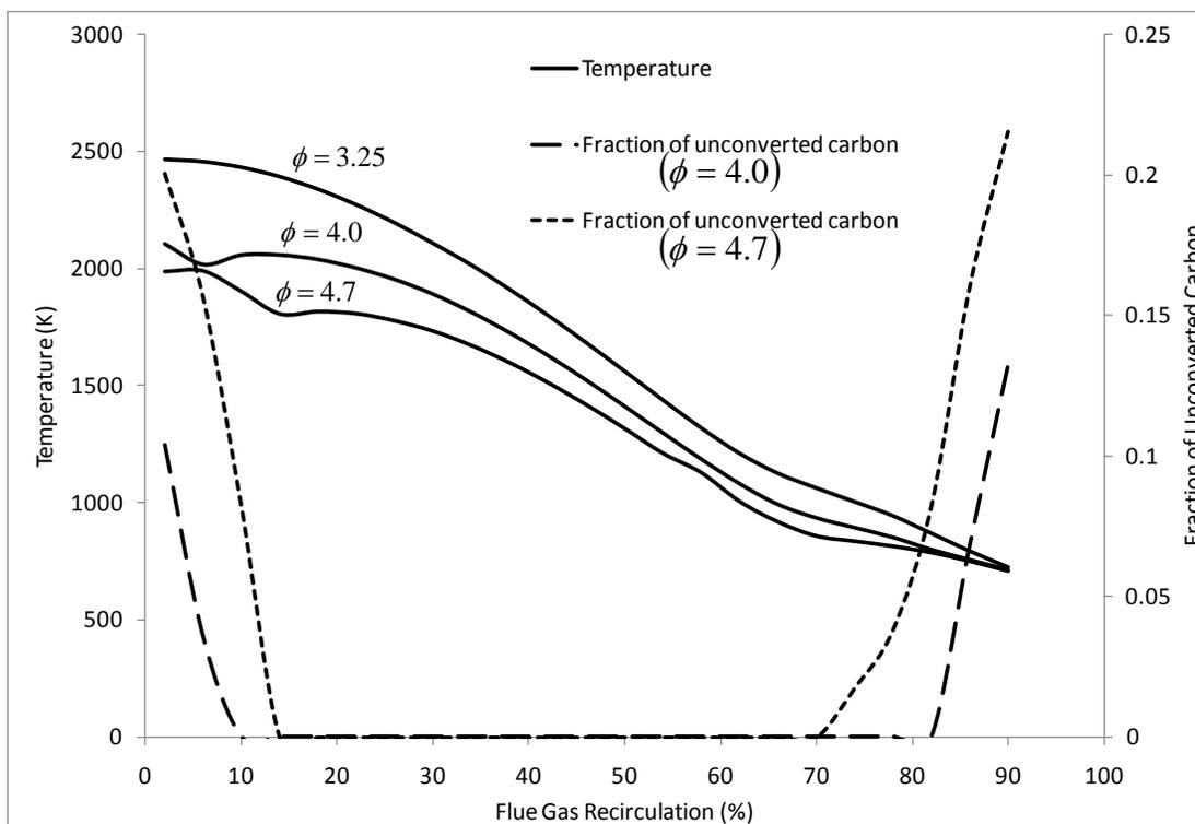
Figure 6-8: Adiabatic reactor temperature vs. percent FGR with flue gas from combustion with pure oxygen.
