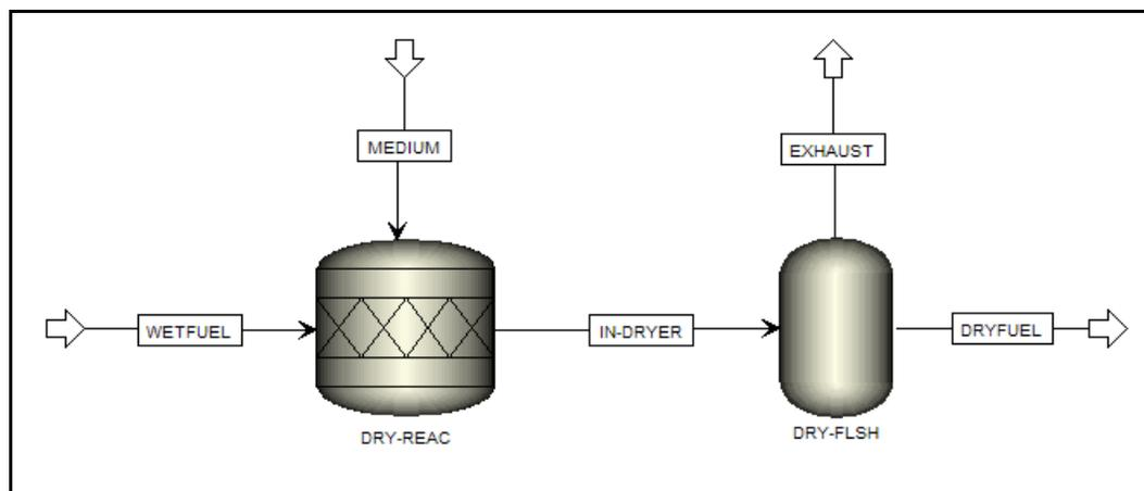
Figure 3-5: Aspen Plus<sup>®</sup> flowsheet of the dryer model.
