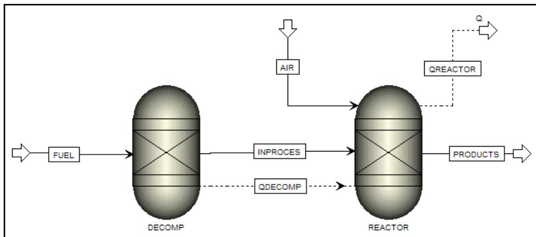
Figure 3-2: Aspen Plus<sup>®</sup> flowsheet of the non-adiabatic gasification model.
