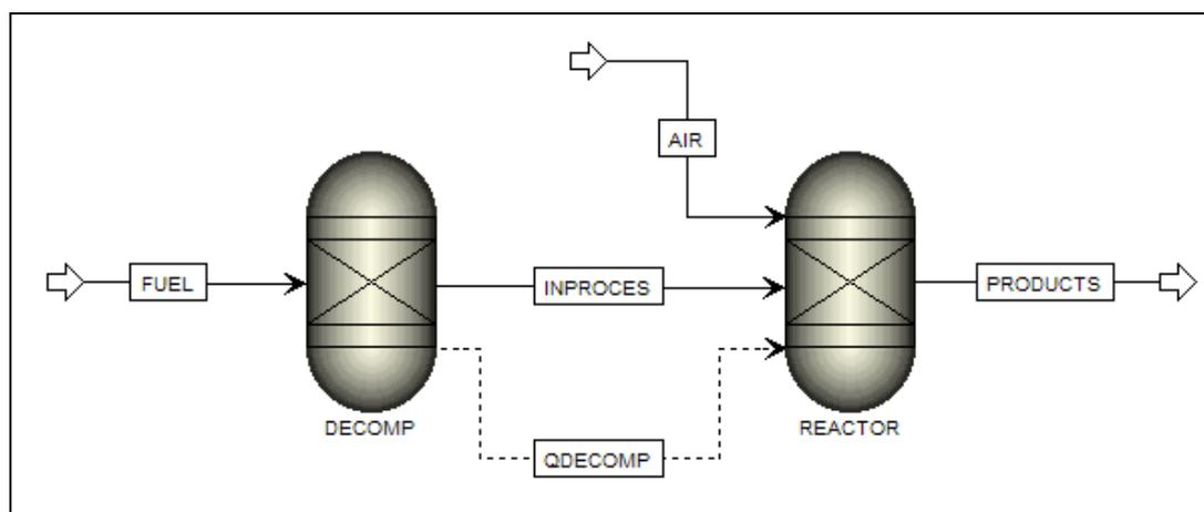
Figure 3-1: Aspen Plus<sup>®</sup> flowsheet of the adiabatic gasification model.
