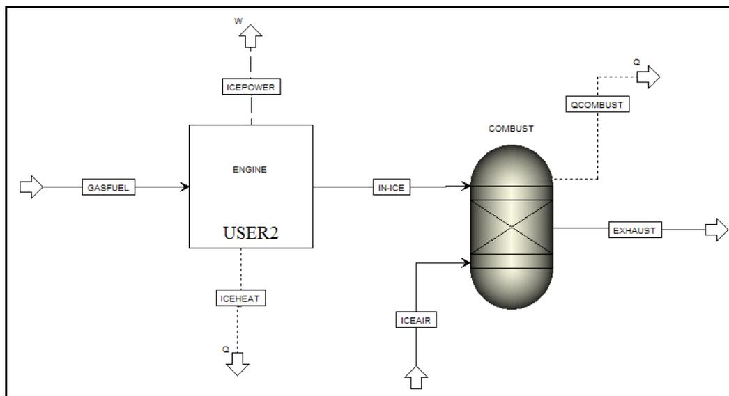
Figure 4-4: Aspen Plus<sup>®</sup> flowsheet of internal combustion engine model.
