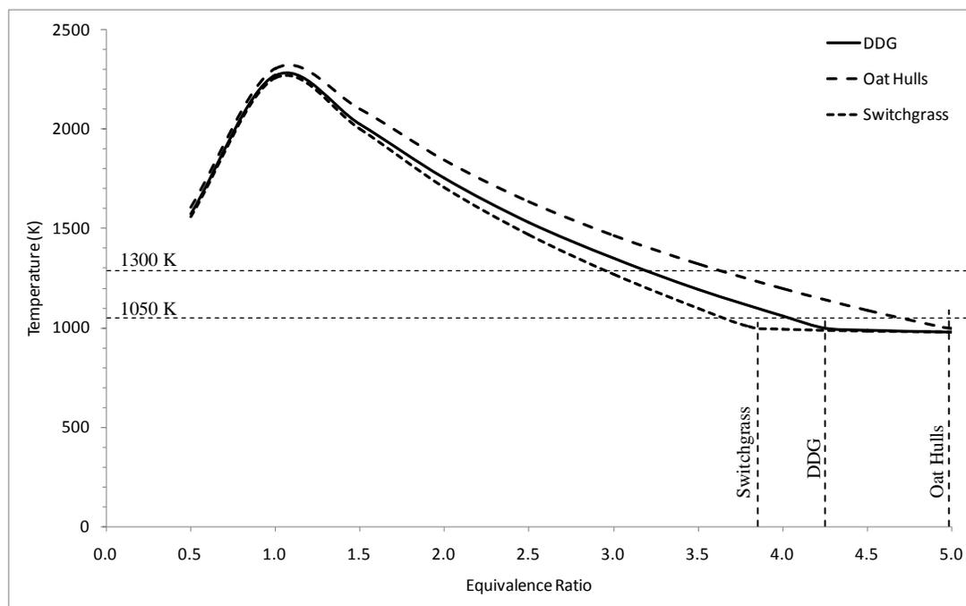
Figure 5-8: Adiabatic reactor temperatures of the biomass fuels.
