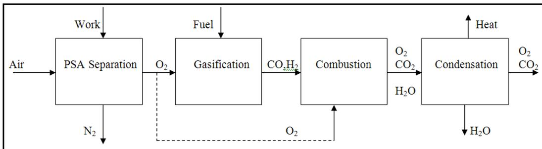
Figure 6-1: Simplified oxyburn gasification plant.
