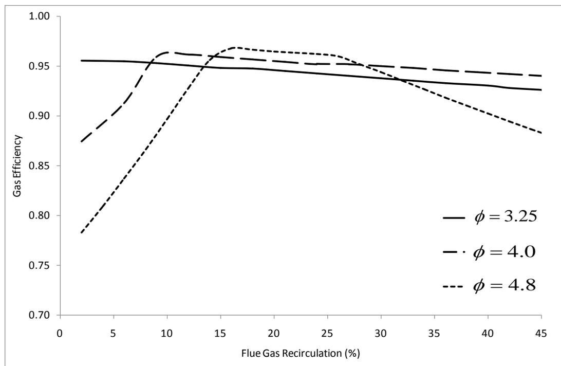
Figure 6-12: Gas efficiency vs. percent FGR with flue gas from combustion with air.
