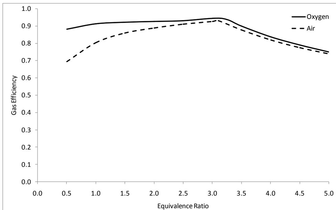
Figure 6-6: Gas efficiencies of coal oxidized by oxygen and air.
