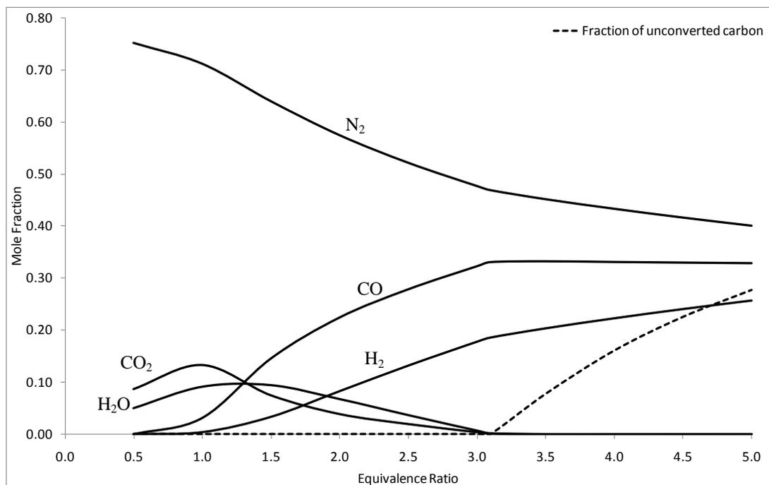
Figure 5-1: Producer gas composition - coal.
