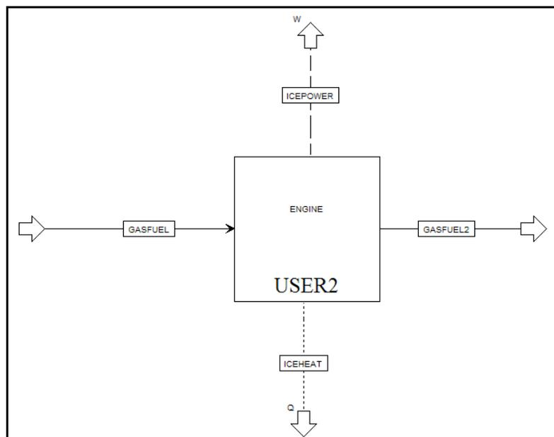
Figure 4-2: Aspen Plus<sup>®</sup> flowsheet of the custom engine model.
