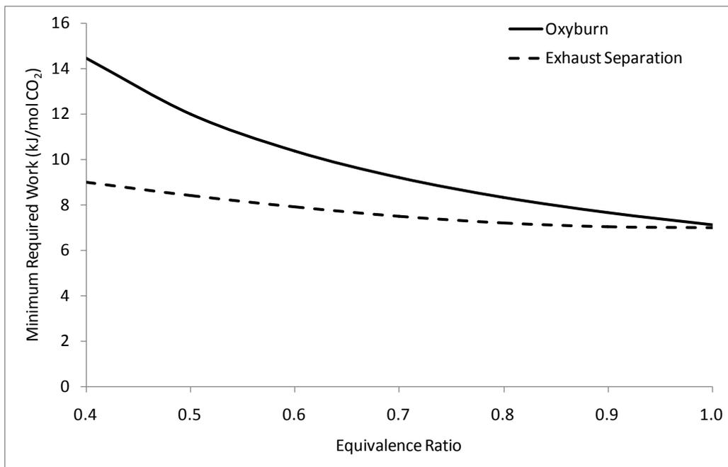
Figure 6-3: Minimum work required for gas separation processes to capture CO<sub>2</sub>.
