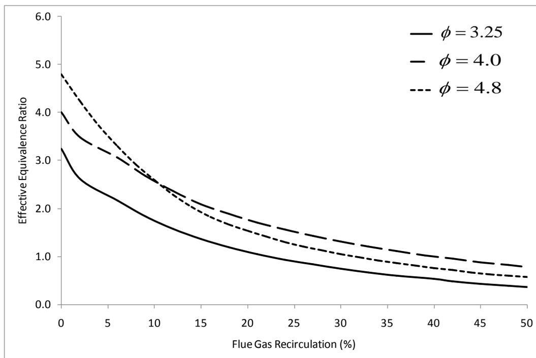
Figure 6-13: Effective equivalence ratio vs. percent FGR with flue gas from combustion with air.
