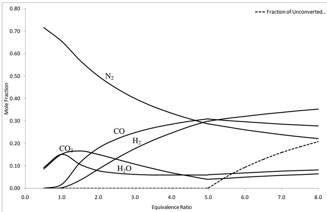
Figure 5-5: Producer gas composition - oat hulls.
