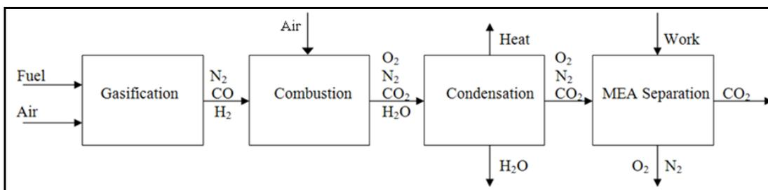
Figure 6-2: Simplified air-gasification plant.
