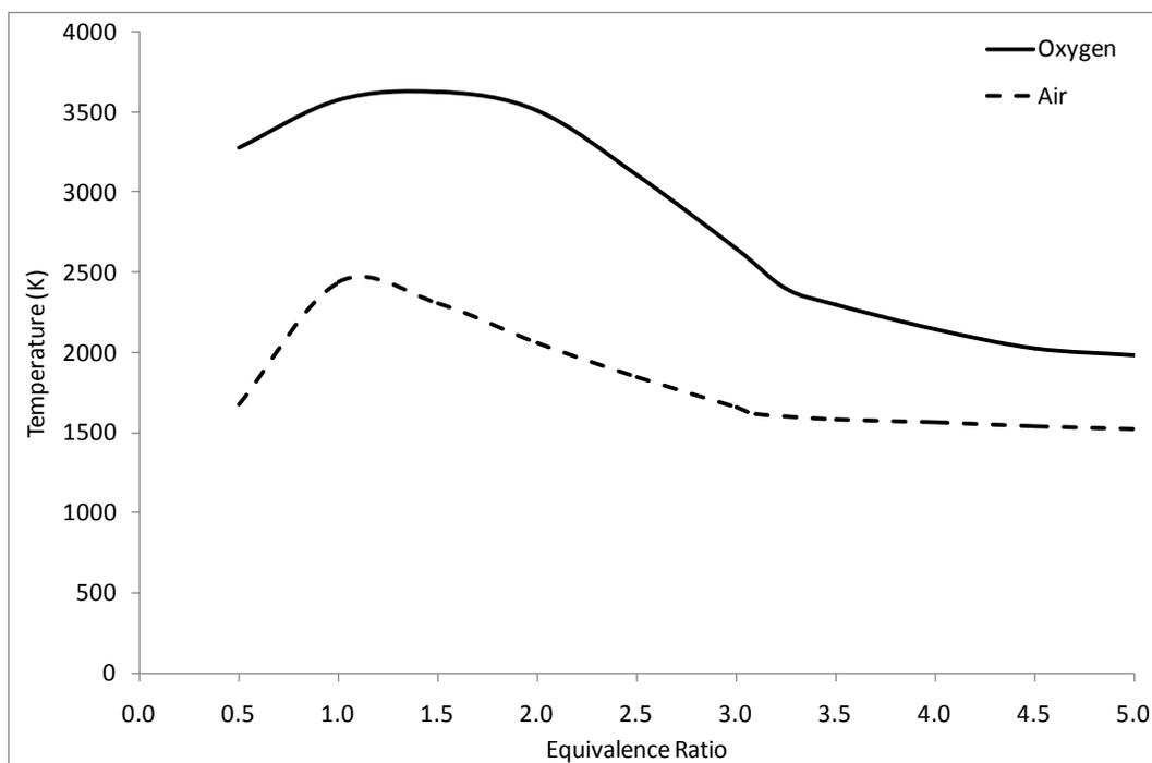
Figure 6-4: Adiabatic reactor temperatures of coal oxidized by oxygen and air.
