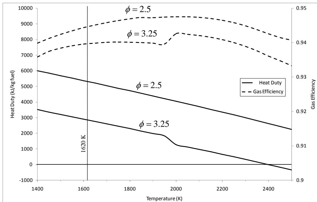
Figure 6-7: Heat duty and gas efficiency vs. temperature for coal oxidized by oxygen.
