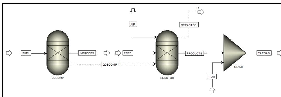
Figure 3-4: Aspen Plus<sup>®</sup> flowsheet of the gasification model with tar addition.
