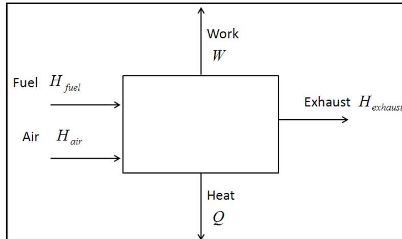
Figure 4-5: Simplified energy flow diagram of an internal combustion engine.
