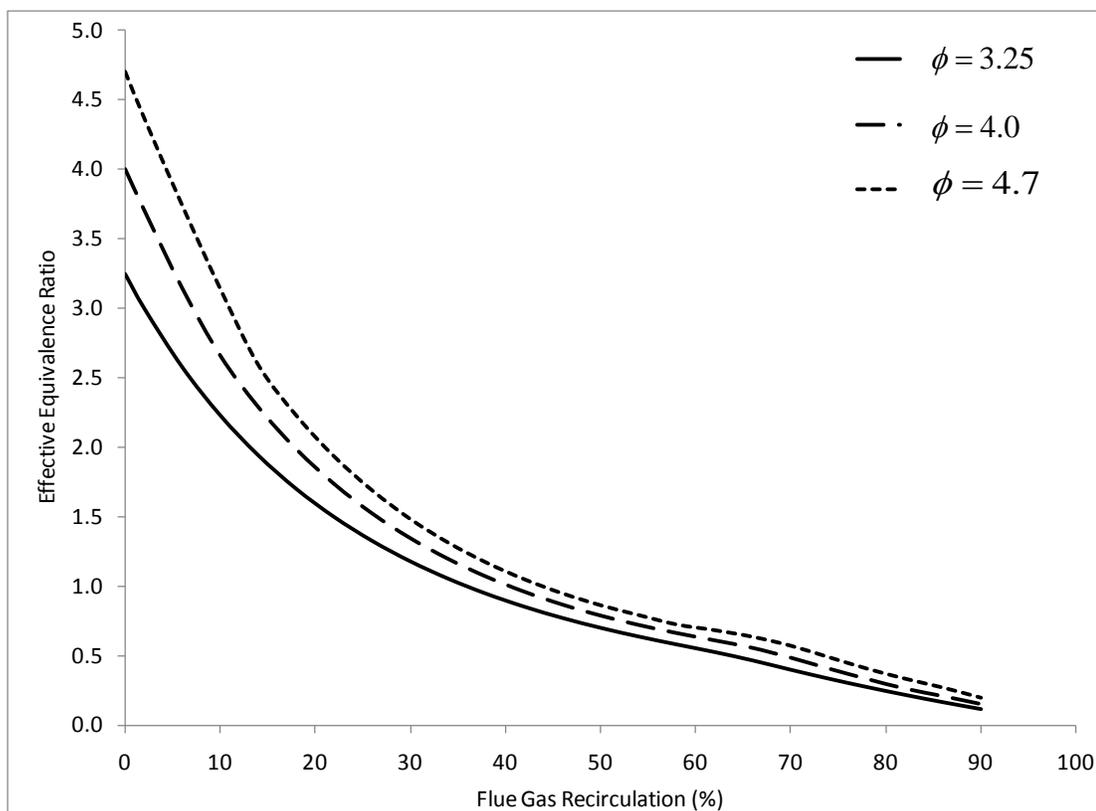
Figure 6-10: Effective equivalence ratio vs. percent FGR with flue gas from combustion with pure oxygen.
