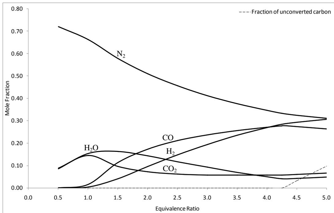
Figure 5-4: Producer gas composition - DDG.
