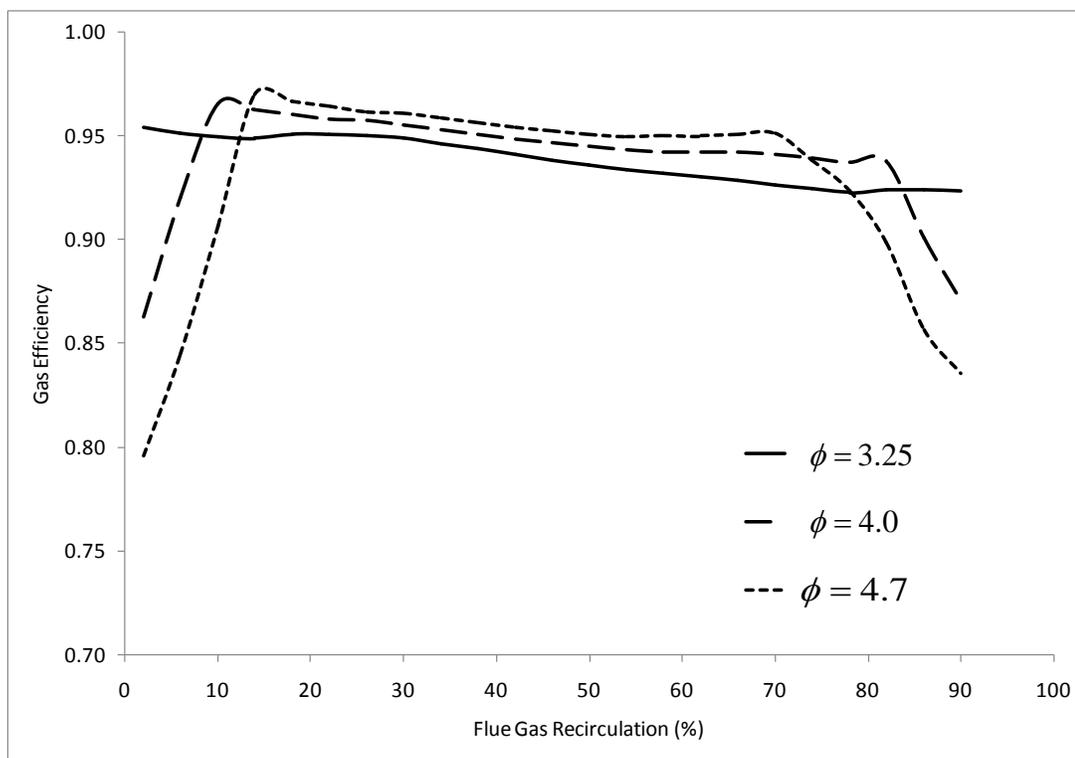
Figure 6-9: Gas efficiency vs. percent FGR with flue gas from combustion with pure oxygen.
