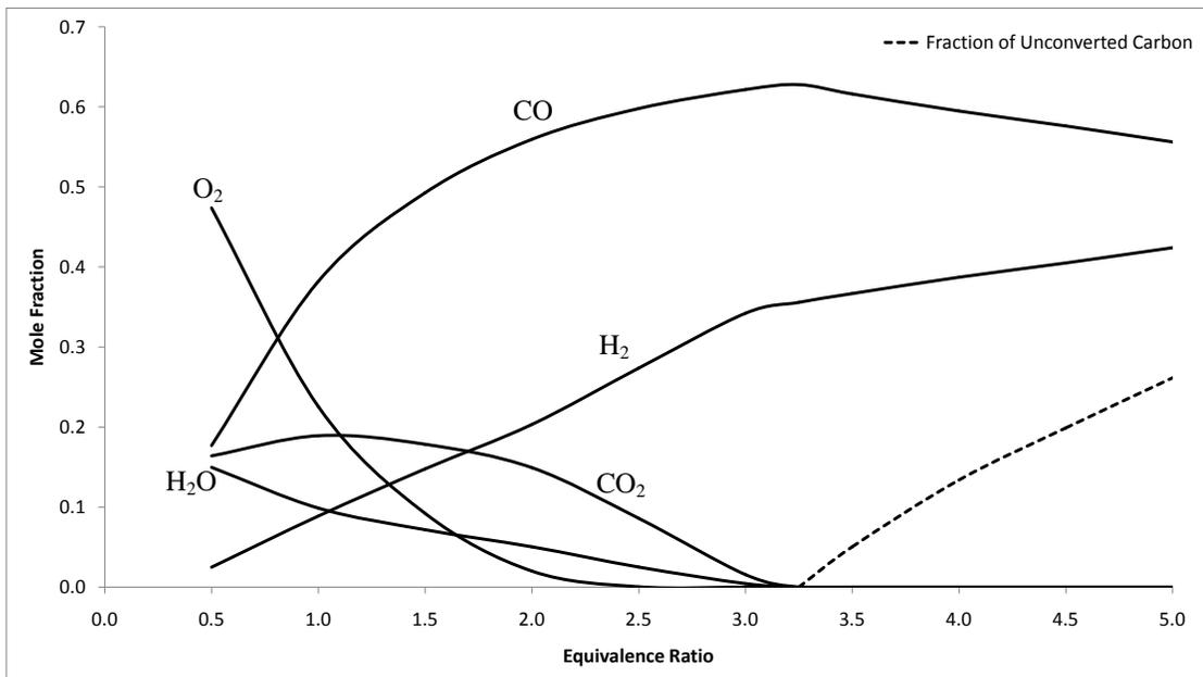
Figure 6-5: Producer gas composition – coal oxidized by pure oxygen.
