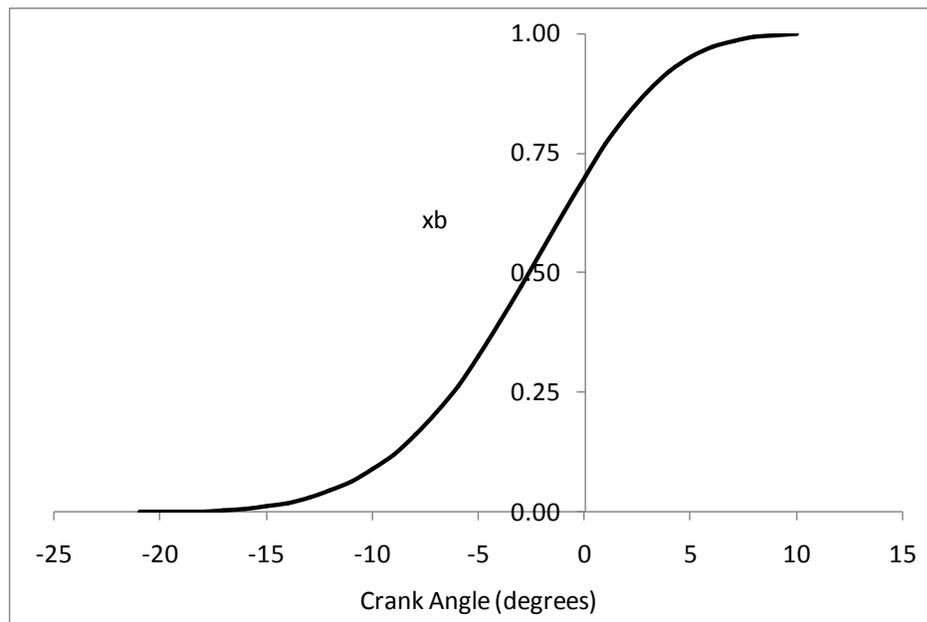
Figure 4-1: Mass burn fraction represented by a typical Wiebe curve.
