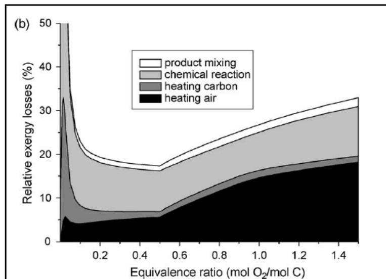
Figure 2-2: Exergy losses of adiabatic carbon reactor vs. equivalence ratio.
