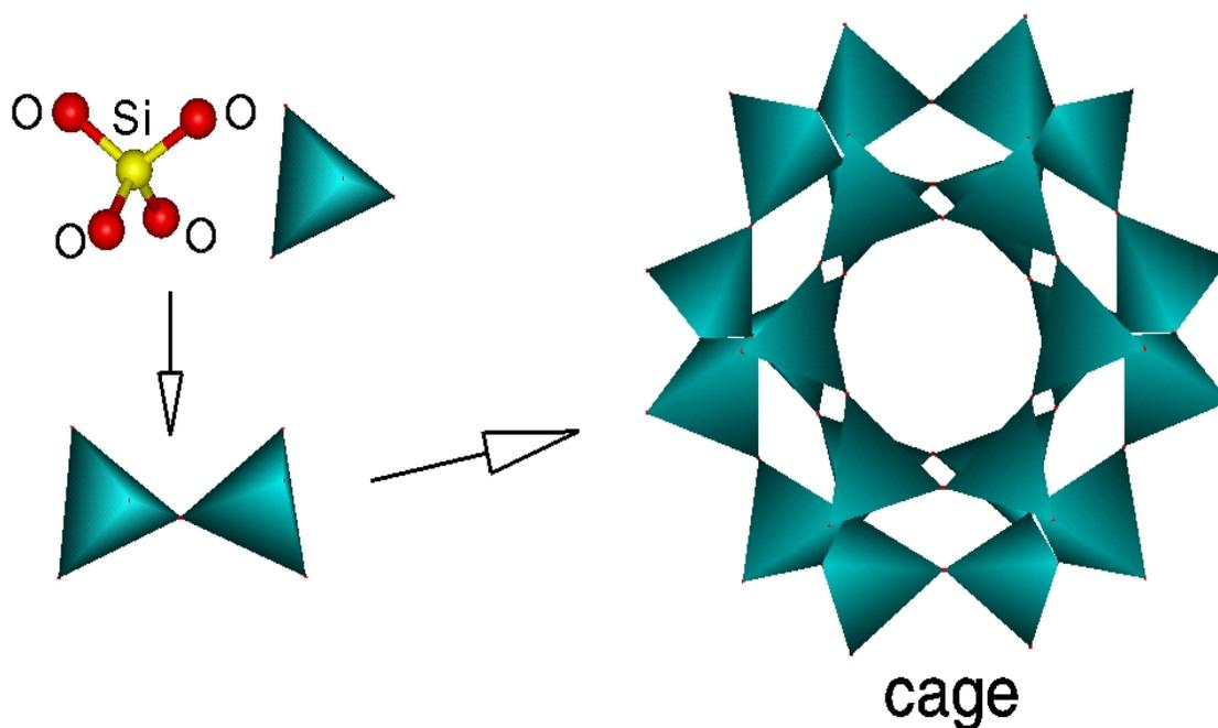
Figure 1.1:  $\text{SiO}_4$  tetrahedron, showing the grouping of formations into larger zeolite structures.
