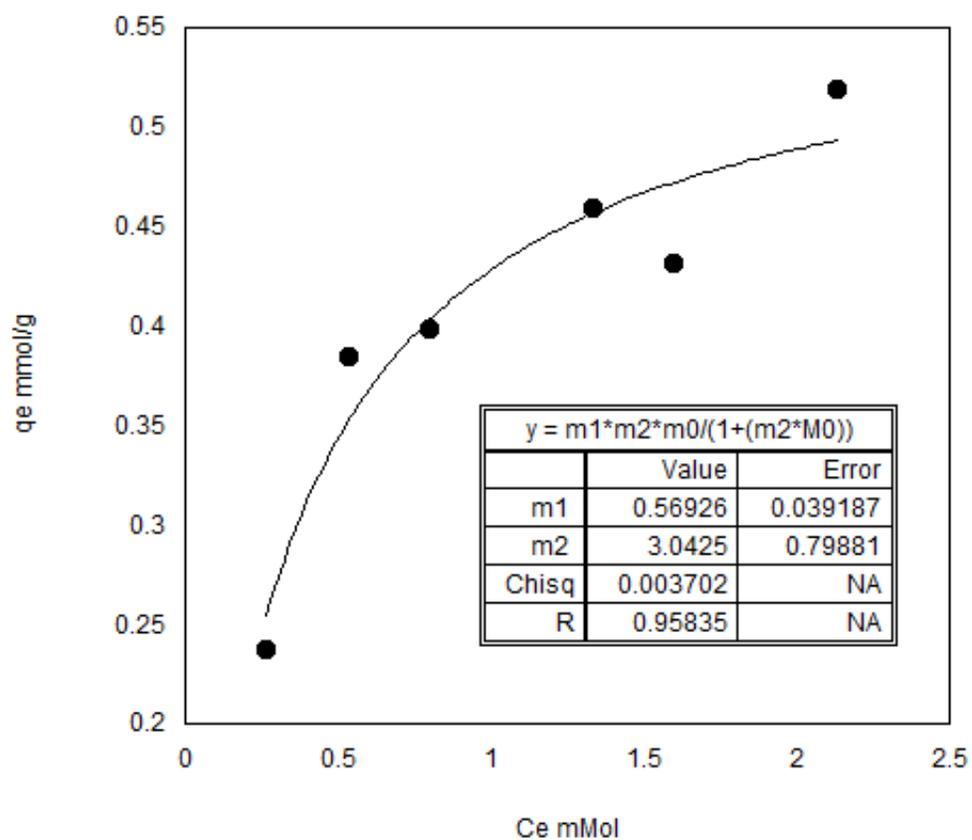
Figure 5.4 Langmuir isotherm fit for Fe<sup>3+</sup> exchanged zeolite
