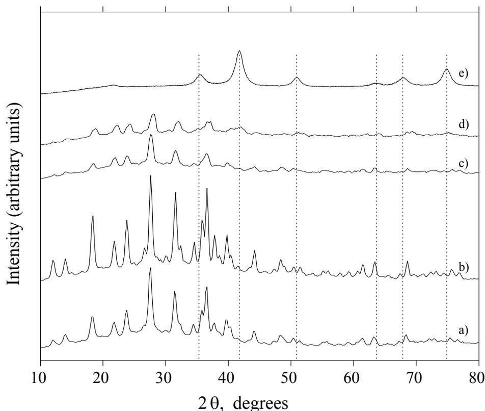
Figure 5.1 Powder X-ray diffraction patterns for a) Y-nano, b) iron oxide/Y-nano-APTES, c) iron oxide/Y-nano-APTES-Fe<sup>3+</sup> and d) iron oxide/Y-commercial-APTES-Fe<sup>3+</sup> and e) iron oxide (Fe<sub>2</sub>O<sub>3</sub>) as synthesized. Dashed lines indicate the iron oxide (Fe<sub>2</sub>O<sub>3</sub> and/or Fe<sub>3</sub>O<sub>4</sub>) reflections.
