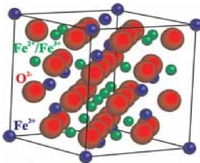
Figure 1.5 Magnetite crystal structure, with Fe<sup>2+</sup> and Fe<sup>3+</sup>
