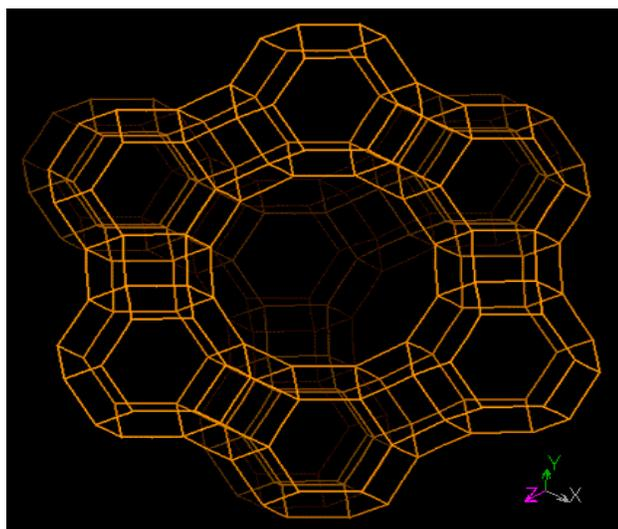
Figure 1.3 Picture of zeolite Y Faujasite type structure.
