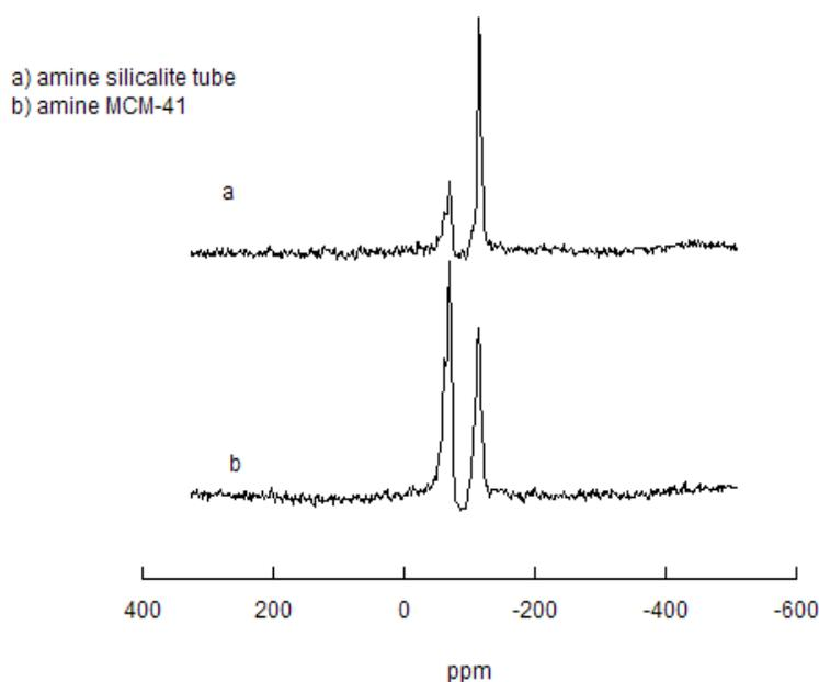
Figure 2.6 <sup>29</sup>Si MAS NMR spectra for a) amine functionalized tubes and b) MCM-41 tubes.
