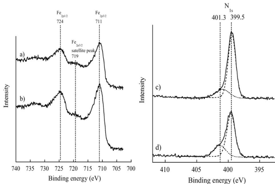
Figure 3.3. XPS spectra of the Fe region of the XPS spectra for a) iron oxide/Y-Zeolyst-APTES and b) iron oxide/Y-nano-APTES. XPS spectra of the  $\text{N}_{1s}$  region of the XPS spectrum for c) iron oxide/Y-Zeolyst-APTES and d) iron oxide/Y-nano-APTES
