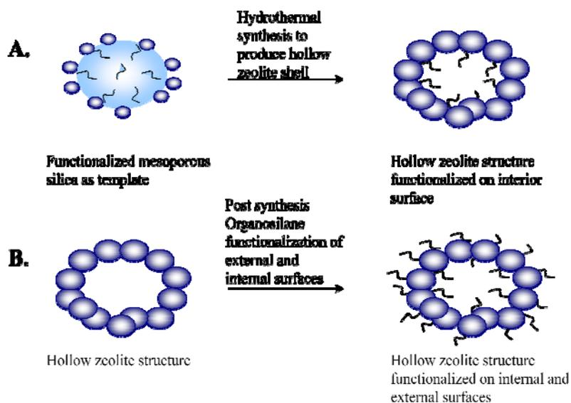
Figure 2.2 Scheme for making hollow tubes and functionalized hollow zeolite tubes
