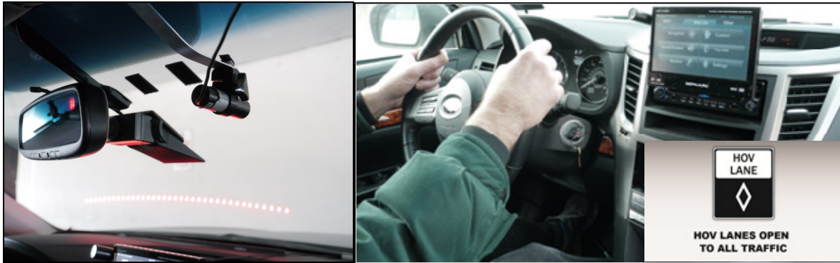
Figure 2. Visual component of EEBL warning reflected in windshield (left), view of default display screen on center stack (right) and example of driver assistance message (inset)
