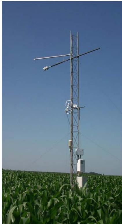
Figure 8. A photograph of the CSAT3 and LI7500 station.
