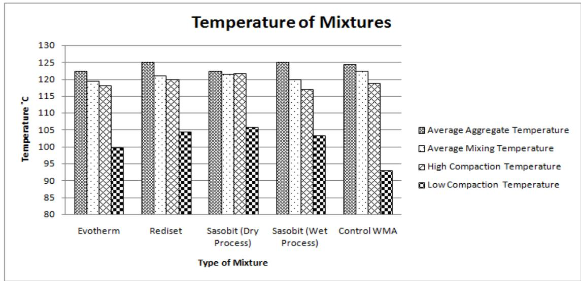
Figure 8: Comparison of the different temperatures of samples
