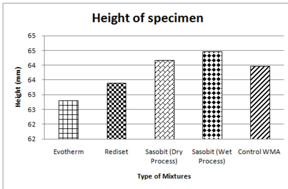
Figure 12: Average height attained by different specimens
