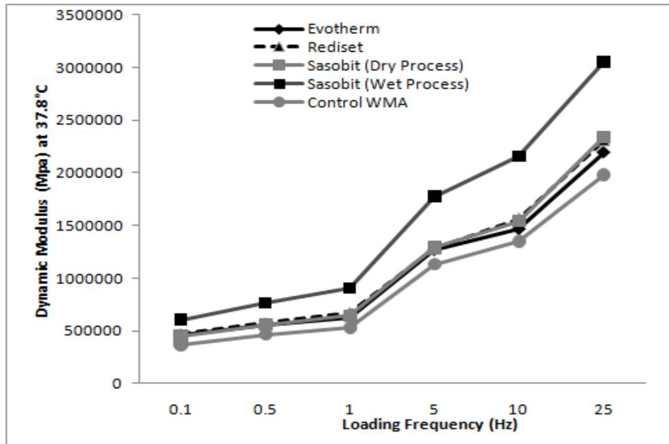
Figure 17: Dynamic modulus of the specimen at 37.8°C
