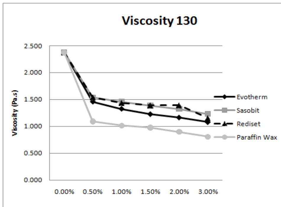
Figure 4: Viscosity of the binder at 130°C
