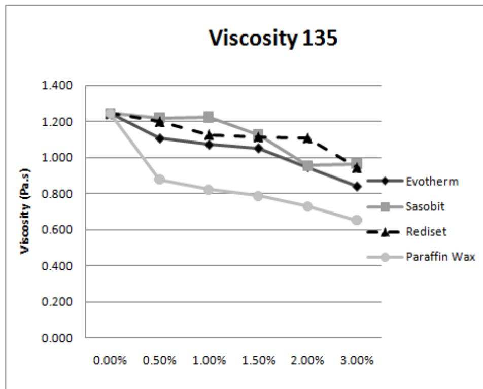
Figure 3: Viscosity of the binder at 135°C
