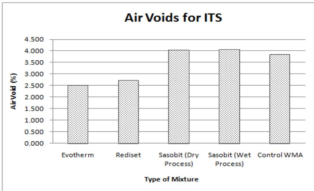
Figure 10: Comparison of the airvoids of different samples.
