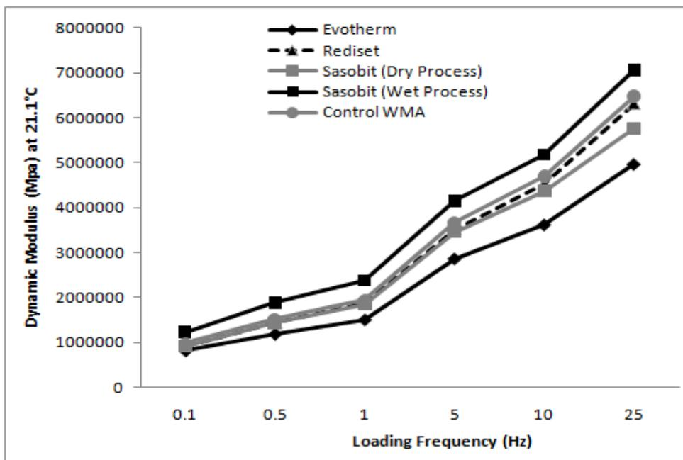
Figure 16: Dynamic modulus of the specimens at 21.1°C
