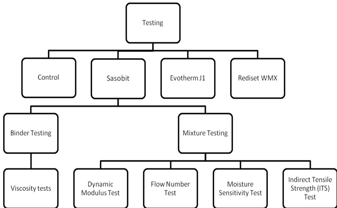
Figure 2: Flow chart of the list of experiments performed
