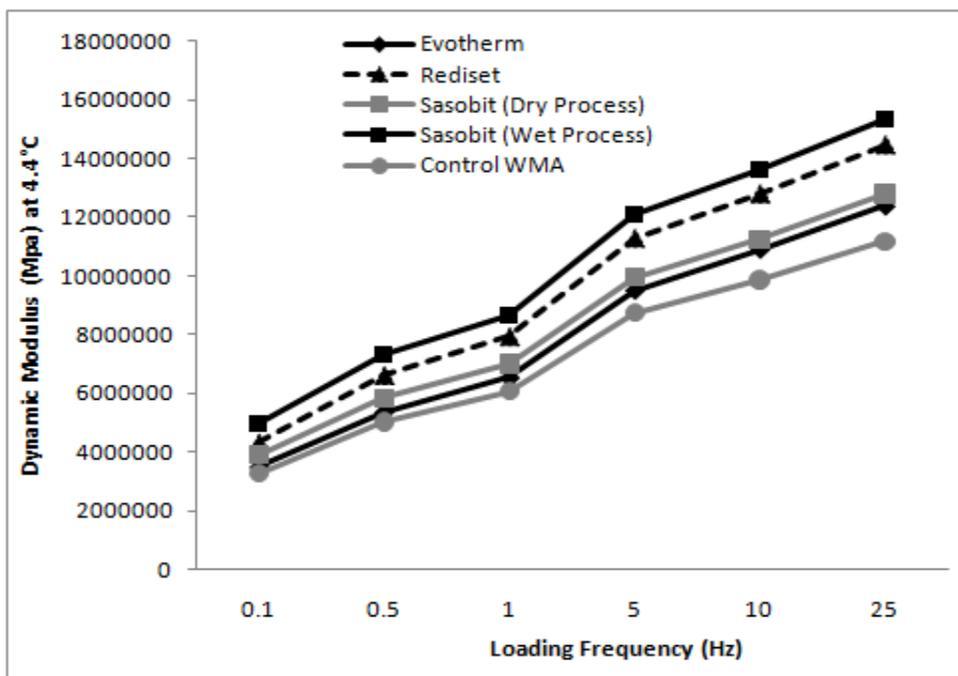
Figure 15: Dynamic modulus of the additives at 4.4°C
