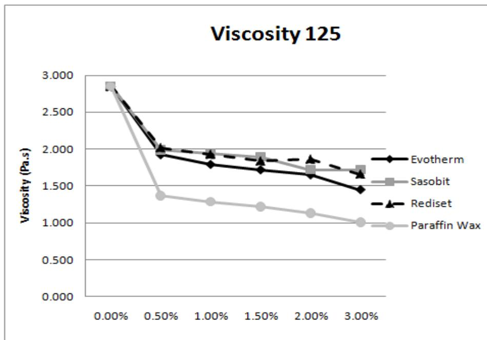
Figure 5: Viscosity of the binder at 125°C
