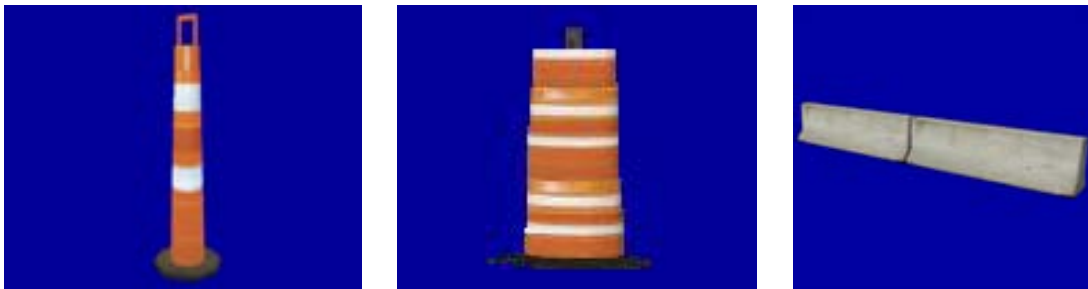
Figure 4. Three different barrier types evaluated in this study: 42-inch channelizer, drum, and concrete barrier
