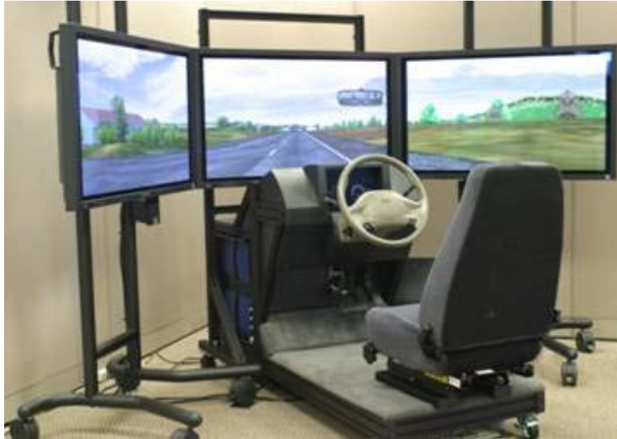
Figure 2. The National Advanced Driving Simulator (NADS) MiniSim
