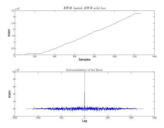
Figure 2.6: Actual KWH, its estimate and autocorrelation of model (8)
