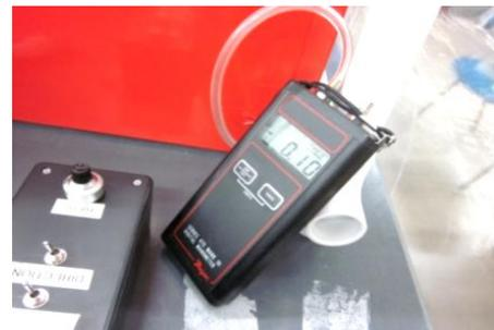
Figure A6. The pressure inside the cabinet.
