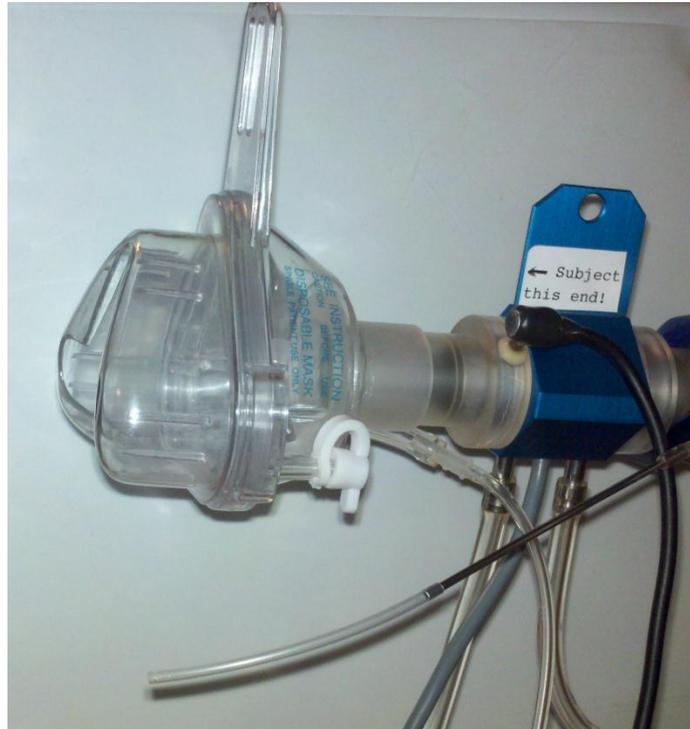
Pictured above is the nasal mask, pneumotachograph, and air pressure sensing tubing portion of the PERCI-SAR system used to collect the aerodynamic measurements including oral pressure, nasal pressure, nasal flow, VP area, and SPL.
