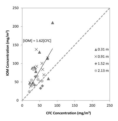
Figure C1 - IOM and CFC concentration data collected for sawdust trials.
