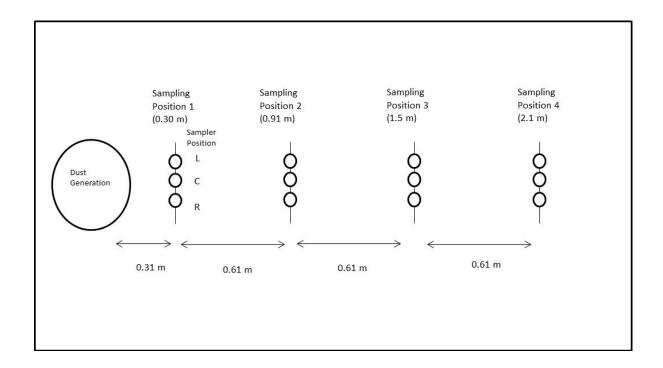
Figure 1 – Overhead view of experimental apparatus.
