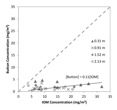
Figure C7 - Button and IOM concentration data collected for glass microbead trials.
