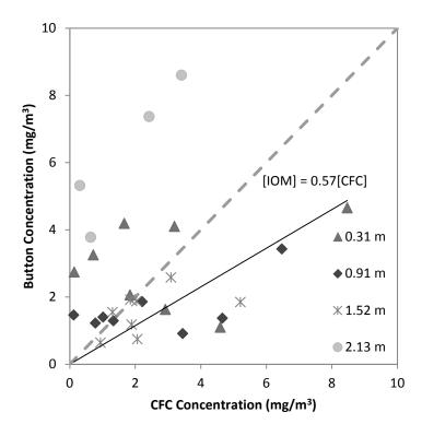
Figure C6 - Button and CFC concentration data collected for glass microbead trials.
