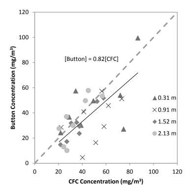
Figure C2 - Button and CFC concentration data collected for sawdust trials.
