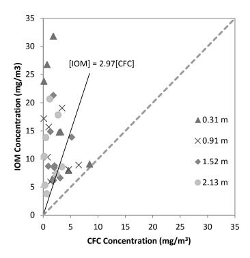
Figure C5 - IOM and CFC concentration data collected for glass microbead trials.
