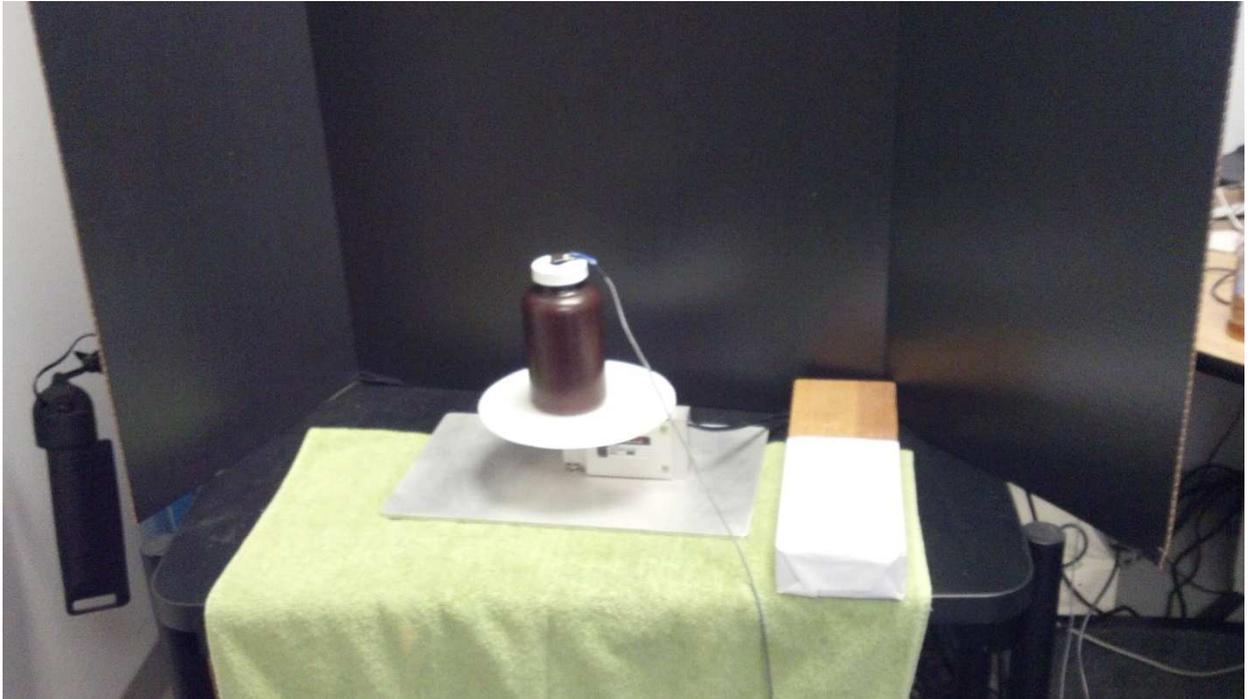
Figure 2-1. Experiment setup with the bottle located on the force plate with the posterboard behind. The board is moved to the right or left of the force plate based on the dominant hand of the subject.
