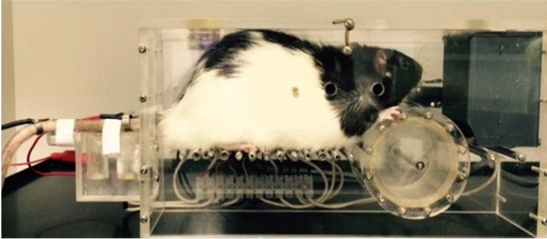
Figure 1. Photograph of a subject in the conditioning task apparatus. Animals were situated in a Plexiglas box and responses were made by turning a small running wheel 22.5°. Tail movement was restricted using medical tape strips. The unconditioned stimulus was delivered through metal floor rungs inside the box and metal rings placed on the tail.
