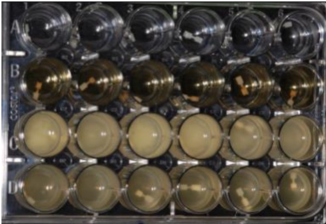
Figure 6: Pilot study aging solutions and the dumbbell-shaped specimens in a 24-well plate
