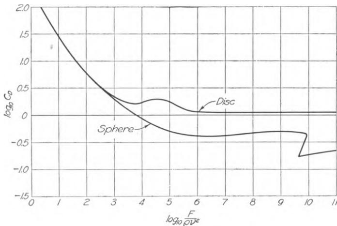
FIG. 8. VARIATION OF  $C_D$  WITH  $\frac{F}{\rho v^2}$  FOR SPHERES AND DISCS.
