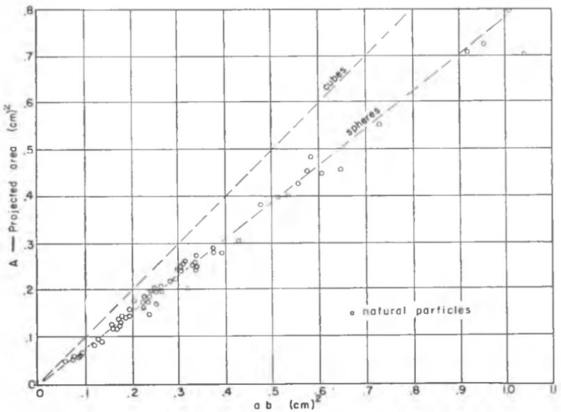
FIG. 2. RELATIONSHIP BETWEEN MAXIMUM PROJECTED AREA AND  $ab$ .
