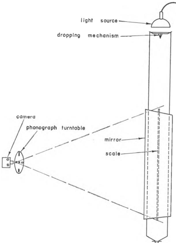
FIG. 1. SCHEMATIC DIAGRAM OF EQUIPMENT FOR MEASURING FALL VELOCITY.
