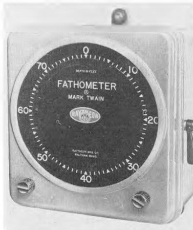
FIG. 1. RED LIGHT DEPTH INDICATOR (RAYTHEON TYPE DE-111)
