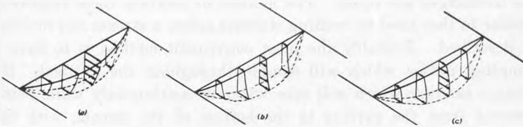
FIG. 3.—VELOCITY AND SEDIMENT DISTRIBUTION IN A FLOWING STREAM.
