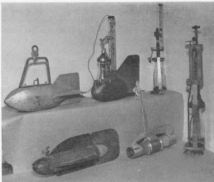
FIG. 4.—A NUMBER OF FORMS OF SUSPENDED-SEDIMENT SAMPLERS.
