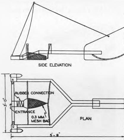
FIG. 2.—BED-LOAD SAMPLER OF THE PRESSURE-DIFFERENCE TYPE DEVELOPED BY THE HYDRAULIC STRUCTURES BUREAU OF THE DUTCH GOVERNMENT.
