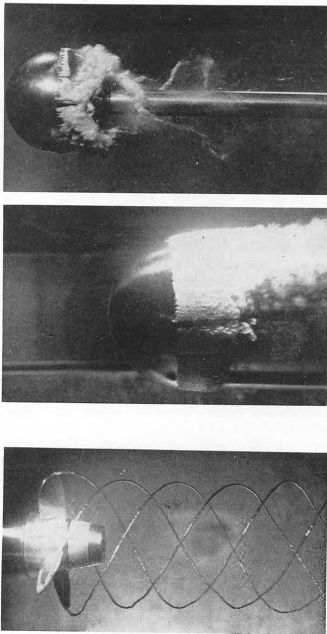
FIG. 10. CAVITATION PHOTOGRAPHY BY ELECTRONIC FLASH, COURTESY OF THE ORDNANCE RESEARCH LABORATORY, STATE COLLEGE, PENNSYLVANIA
