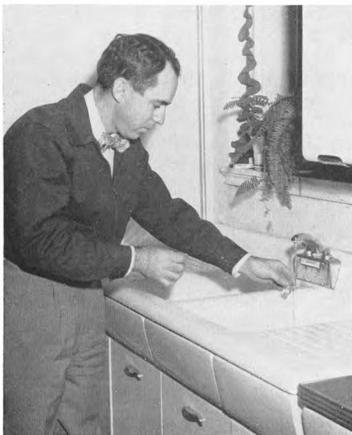
FIG. 11d. AFTER THE LEAK IS REPAIRED, WATER SAMPLES ARE ANALYZED TO ASSURE THAT THE RADIOIODINE IS BELOW THE MAXIMUM PERMISSIBLE CONCENTRATION FOR DRINKING WATER. MAXIMUM PERMISSIBLE CONCENTRATIONS OF RADIOISOTOPES IN WATER ARE PUBLISHED IN NATIONAL BUREAU OF STANDARDS HANDBOOK NO. 52, AVAILABLE FROM THE U. S. GOVERNMENT PRINTING OFFICE, WASHINGTON, 25, D.C., PRICE 20 CENTS.
