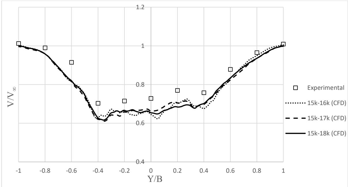
Figure B.2: Comparison of velocity magnitude on lateral line over the flight deck for coarse grid averaged over three different groups of time steps. Velocity and lateral positions are normalized by the freestream velocity and the ship's beam, respectively.
