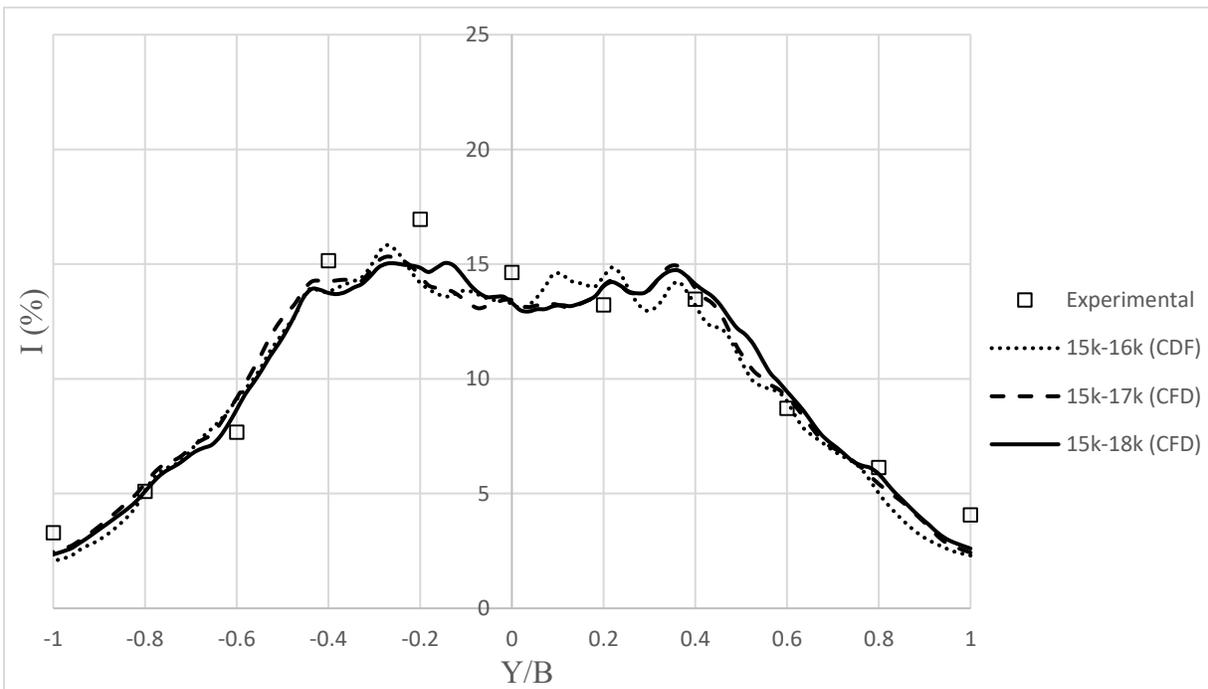
Figure B.5: Comparison of average turbulence intensity on lateral line over the flight deck for the coarse grid calculated over three different groups of time steps. Intensity and lateral position are normalized by the free stream velocity and the ship's beam, respectively.
