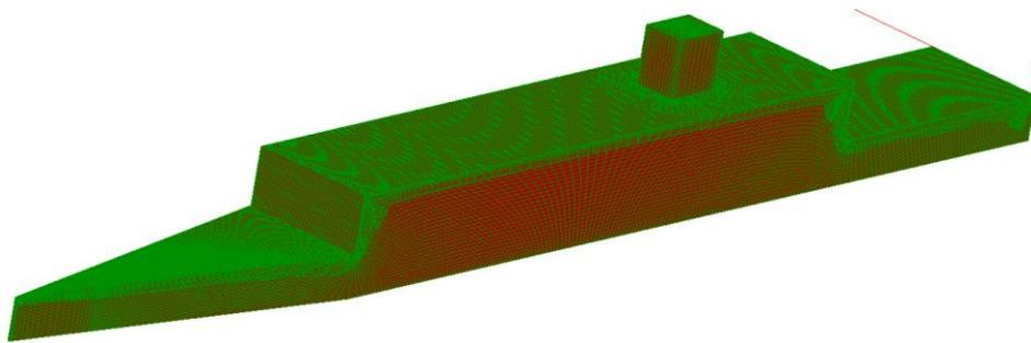
Figure A.2: Overset grid system used to model the surface of SFS2 geometry.
