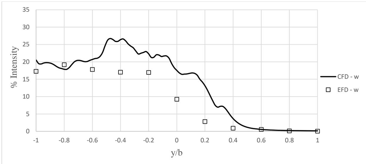
Figure C.4: Comparison of turbulence intensity in the w-direction on lateral line over the flight deck. CFD turbulence intensities were calculated from 9000-15000  $\Delta t^*$ . Turbulence intensity and lateral position are normalized by free stream velocity and the ship's beam, respectively.
