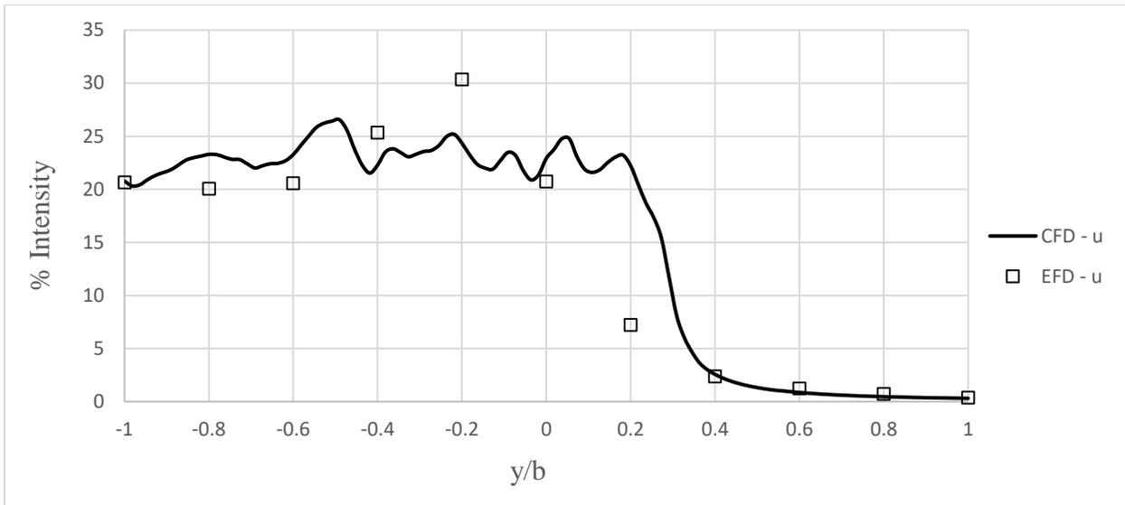
Figure C.2: Comparison of turbulence intensity in the u-direction on lateral line over the flight deck. CFD turbulence intensities were calculated from 9000-15000  $\Delta t^*$ . Turbulence intensity and lateral position are normalized by free stream velocity and the ship's beam, respectively.
