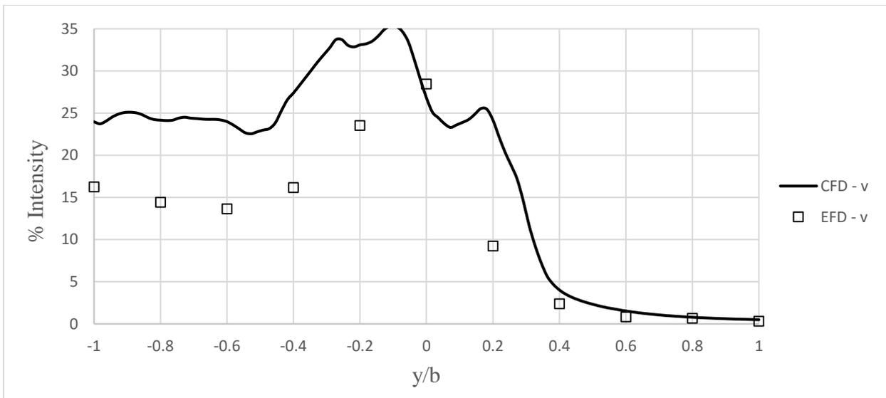
Figure C.3: Comparison of turbulence intensity in the v-direction on lateral line over the flight deck. CFD turbulence intensities were calculated from 9000-15000  $\Delta t^*$ . Turbulence intensity and lateral position are normalized by free stream velocity and the ship's beam, respectively.
