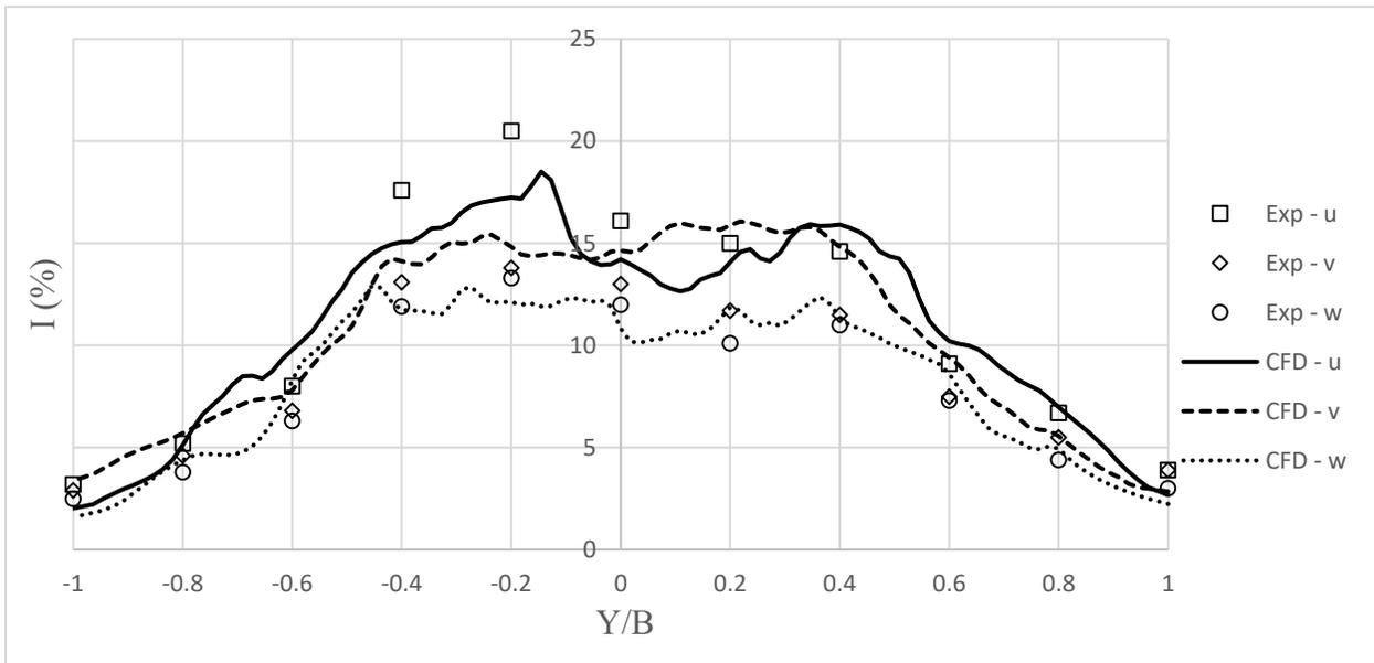
Figure B.7: Comparison of turbulence components on lateral line over the flight deck for the coarse grid. CFD RMS values were calculated from 15000-18000  $\Delta t^*$ . Turbulence intensity and lateral position are normalized by free stream velocity and the ship's beam, respectively.
