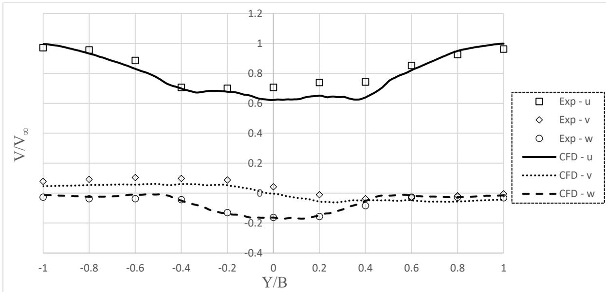
Figure B.4: Comparison of velocity components on lateral line over the flight deck for the fine grid. CFD velocities were averaged from 15000-18000  $\Delta t^*$ . Velocity and position are normalized by the freestream velocity and the ship's beam, respectively.
