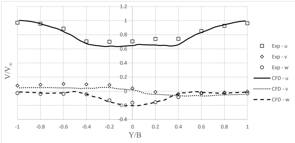
Figure B.3: Comparison of velocity components on lateral line over the flight deck for the coarse grid. CFD velocities were averaged from 15000-18000  $\Delta t^*$ . Velocity and position are normalized by the freestream velocity and the ships beam, respectively.
