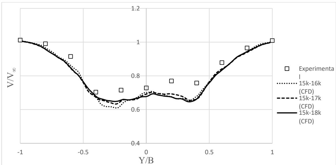
Figure B.1: Comparison of velocity magnitude on lateral line over the flight deck for coarse grid averaged over three different groups of time steps. Velocity and lateral position are normalized by the free stream velocity and the ship's beam, respectively.
