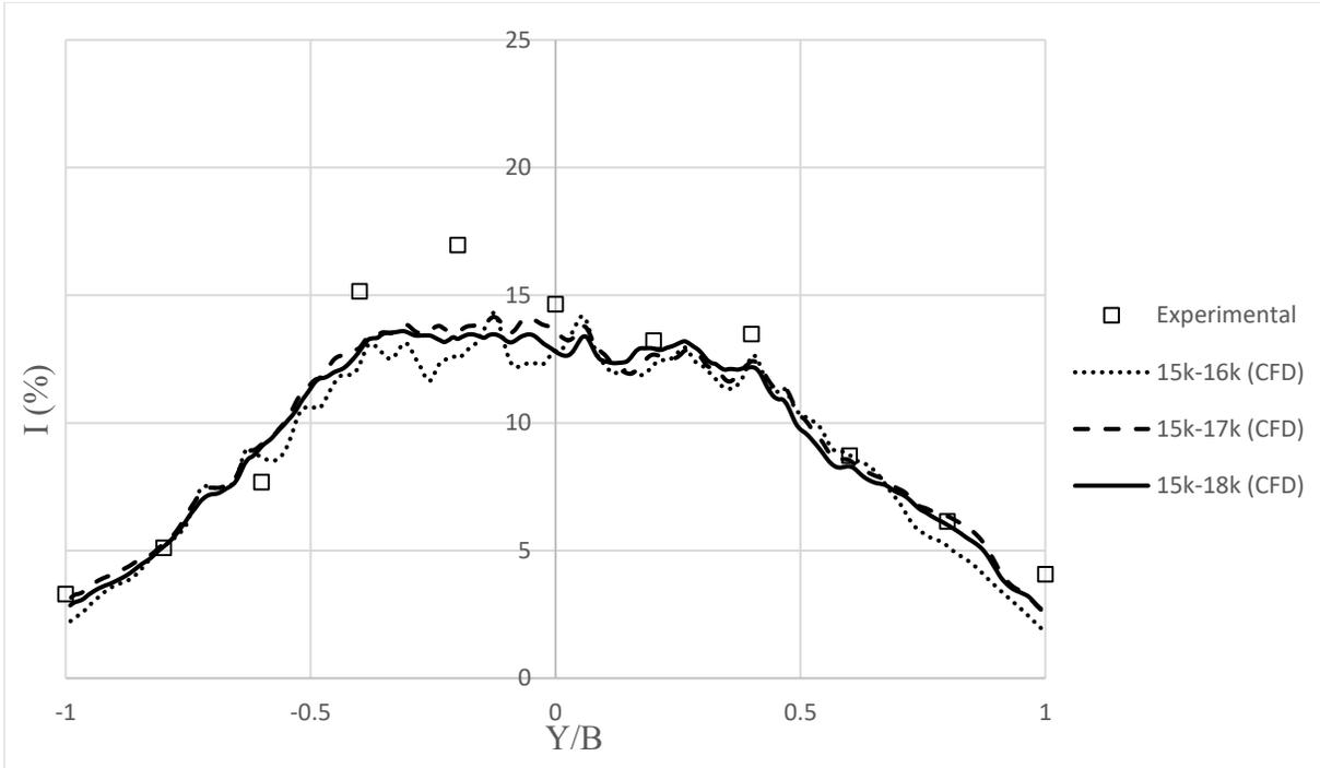
Figure B.6: Comparison of average turbulence intensity on lateral line over the flight deck for the fine grid calculated over three different groups of time steps. Turbulence intensity and lateral position are normalized by free stream velocity and the ship's beam, respectively.
