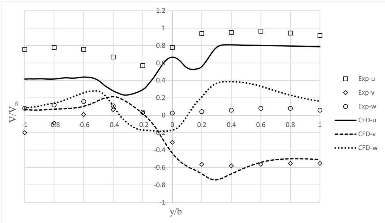
Figure C.1: Comparison of velocity components on lateral line over the flight deck. CFD velocities were averaged from 9000-15000  $\Delta t^*$ . Velocity and position are normalized by the freestream velocity and the ships beam, respectively.
