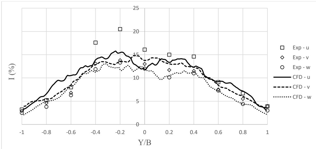
Figure B.8: Comparison of turbulence intensity components on lateral line over the flight deck for the fine grid. CFD RMS values were calculated from 15000-18000  $\Delta t^*$ . Turbulence intensity and lateral position are normalized by free stream velocity and the ship's beam, respectively.
