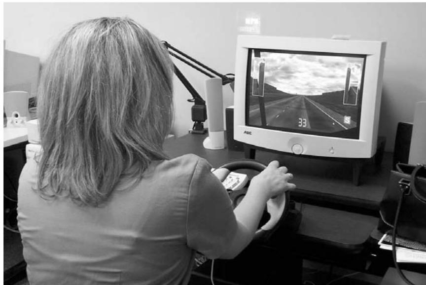
**Figure 1. Level 1 PC Driving Simulator with Joystick Configuration**
