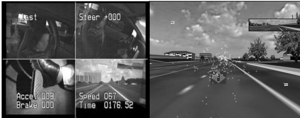
**Figure 1. The image on the left shows a screen capture of the interior of the simulator with brake, accelerator, speed and steering variables overlaid. The image on the right illustrates the diamond in-vehicle sign with the corresponding area of interest (AOI) surrounding it. Fixations for the 4 seconds that the HUD was on prior to the intersection are shown as white dots.**
