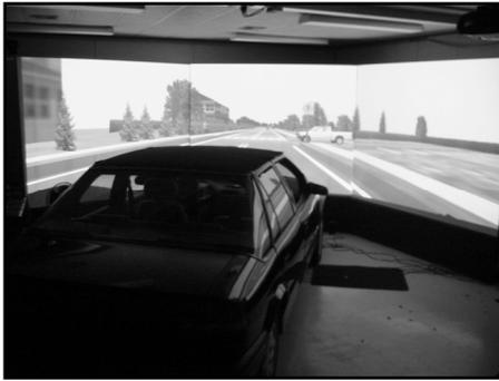
**Figure 2. Driving Simulator, Human Performance Laboratory, UMass**
