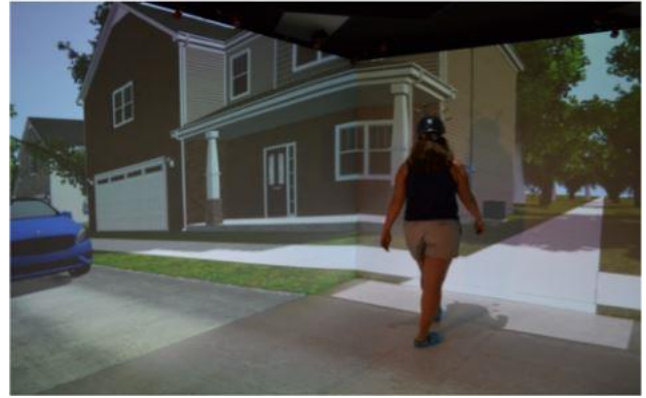
Figure 1: The large-screen (CAVE) pedestrian simulator.
