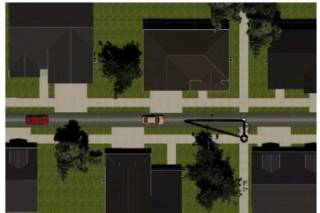
Figure 2: Road distance calculation. Road distance, r , was calculated by multiplying tangent of angle x by distance to the center of the road, d .
