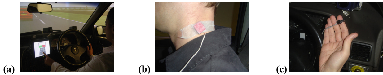
Figure 1. (a) The Phone task, (b) the tactor, (c) the microswitch used for all detection tasks
