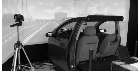
Figure 1. High-fidelity driving simulator and camera setup
