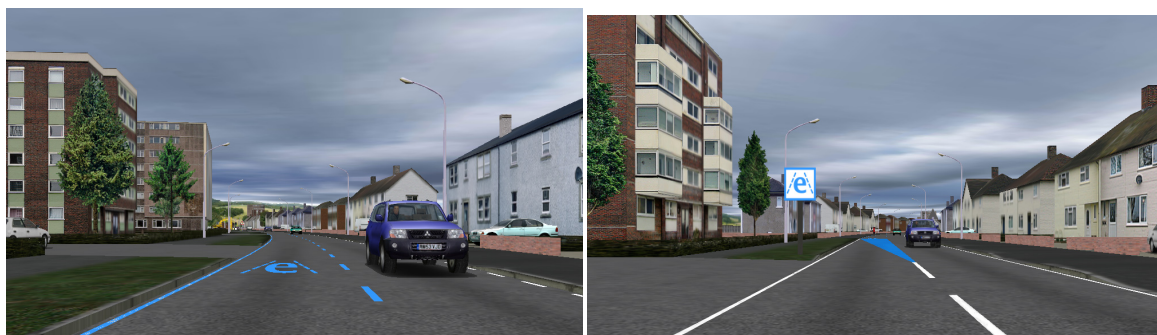
Figure 2. The road markings (left) and sign (right) used to denote the eLane
