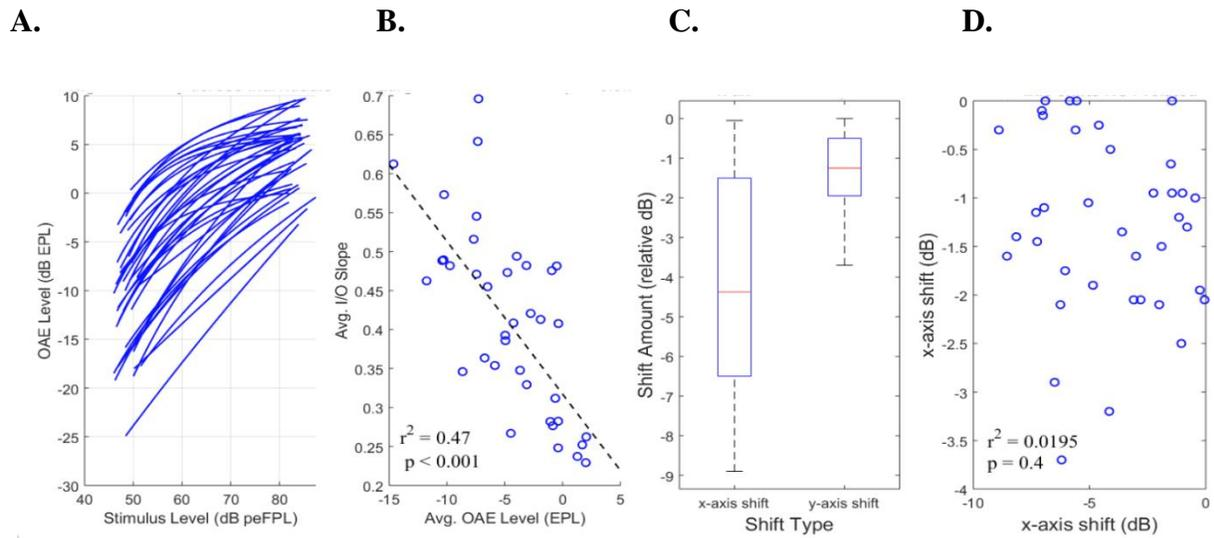
**Figure 5:** Group results. A. High variability in OAE input/output functions seen across 38 subjects, both in overall level and growth rate. B. Higher OAE levels tended to have more compressive growth. C. Shifts along the x-axis were larger and more variable than shifts along the y-axis. D. Shifts along the x- and y- axes were uncorrelated.
