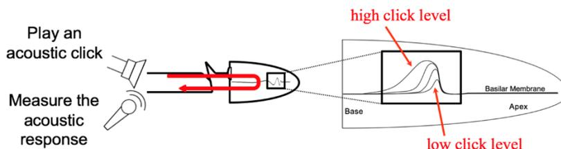
**Figure 2.** Measurement of OAEs. Left side schematic view of the OAE probe (loudspeaker and microphone), ear canal, and cochlea (unrolled). Right side expanded view of BM showing spread of excitation pattern as stimulus level increases.
