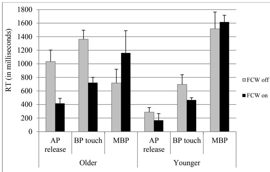
**Figure 1. Reaction times (RTs) in the pedestrian incursion as function of age group and FCW status. RTs were calculated for initial accelerator pedal release (AP release), initial brake depression (BP touch), and brake application time (MBP). Error bars represent standard error estimates**
