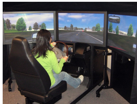
Figure 1. Three-channel quarter cab miniSim
