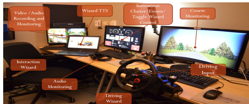
Figure 2: Wizard of Oz Station. Wizard 1 monitors and interacts with participant, Wizard 2 interacts with and manipulates simulation environment.
