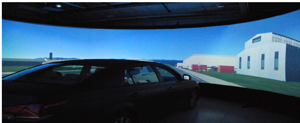
Figure 1: The Driving Simulator is used for experiments on Automated Driving It features a Toyota Avalon chassis and a 270-degree frontal arc seamless curved screen
