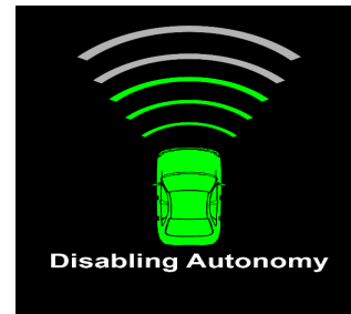
Figure 4. Automation system status indicator on instrument panel. The car icon lights up in green to indicate that the system is on, and turns to grey to when it is off. The arcs in front of the car show when the system is turning on or off, and descriptive text is provided below the vehicle icon
