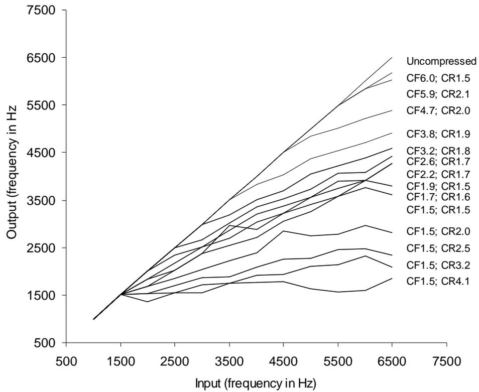
Figure A1. Input/output curves for thirteen different cutoff frequency and compression ratio settings plus the uncompressed condition. Data are shown in frequency (Hz).
