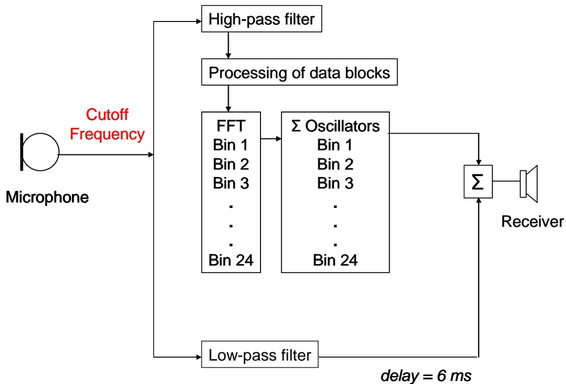
Figure 1.1. A block diagram of the signal processing of a frequency-compression hearing aid (adapted from Simpson et al., 2005).
