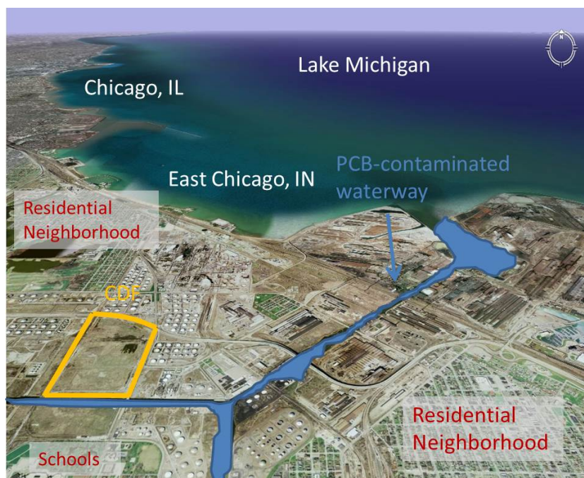
Figure 3 East Chicago, Indiana is bisected by the Indiana Harbor and Ship Canal (IHSC), which is contaminated with high levels of PCBs. A navigational dredging project will place contaminated sediment in the confined disposal facility (CDF).
