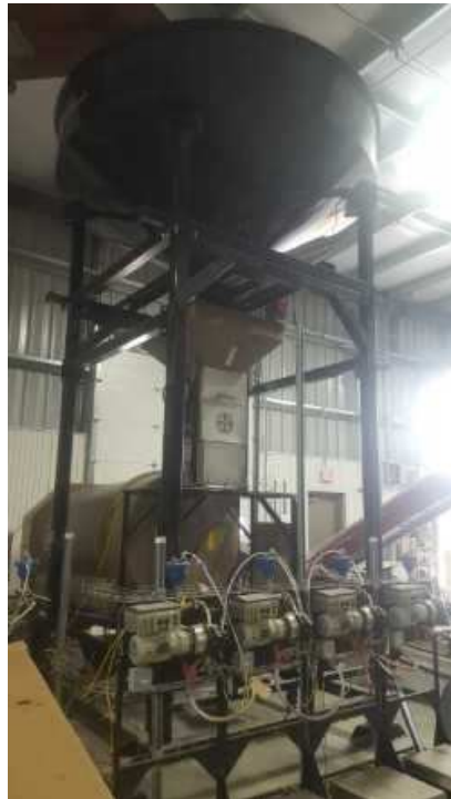
Figure 14. Treater with view of chemical scales in front and bin above which drops the seed down into the treater
