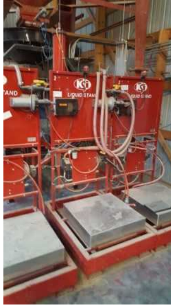
Figure 8. Treatment scales: Ingredient drums are placed on scales to determine amount of liquid remaining in the drum and being taken out during treatment process
