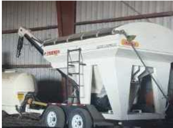
Figure 15. Seed Tender: Used by a farmer to transport seed from suppliers to their farm in bulk. An auger pulls the seed out of the seed tender and loads it into the planter.
