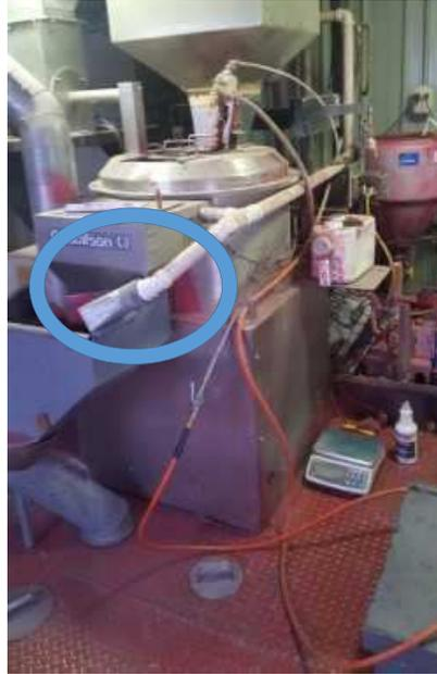
During treatment, water and colorant increase flow ability. The water and colorant are mixed in a slurry tank and then pumped to the application area.
