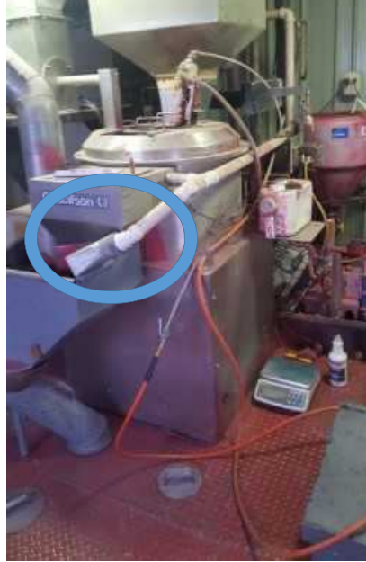
Figure 5. Dust Collector with visible dust around machine and on floor.
