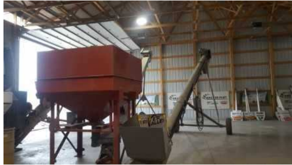
Figure 12. Drying Bin and auger used to fill boxes
