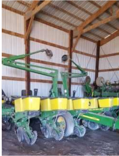
Figure 16. 12-Row Planter: Each individual box is manually filled with seed during planting
