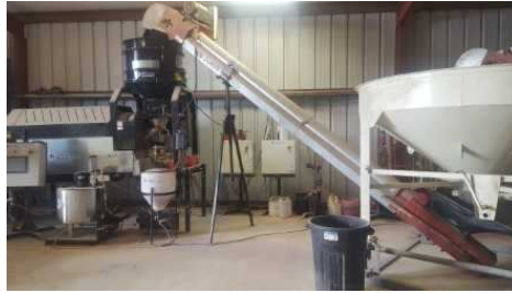
Figure 13. Auger (middle) which drops seed into treater (left)
