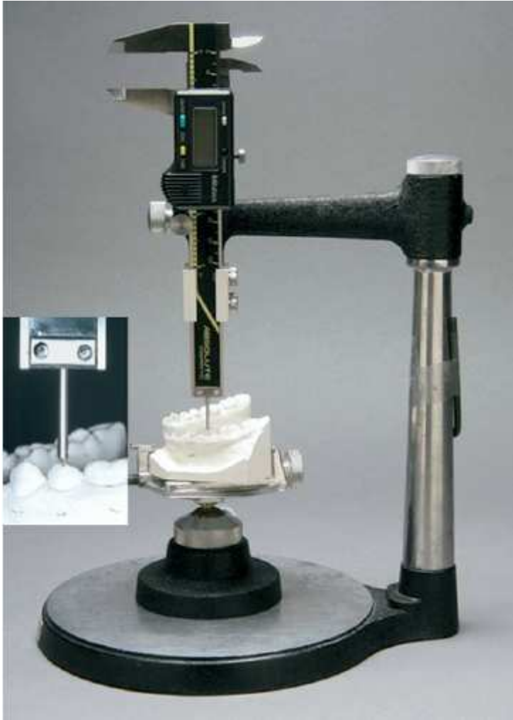
Figure 4: Measuring Apparatus: a digital caliper vertically mounted on a surveyor. The end of the digital caliper is enlarged ( inset ) to show the modification of the caliper arm to allow point contact with the dental cast.
